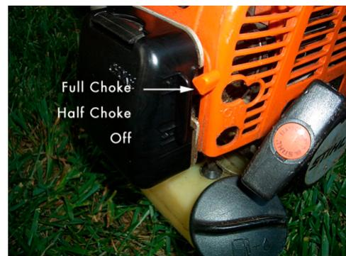
for the first time, move the choke lever on the carburetor from **Off** to **Full Open** (from bottom to top).
